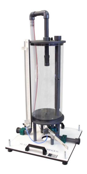
The FL12.1 equipment has been designed for the study of the contraction that occurs when a jet of fluid passes through an orifice. Its design is aimed at making teaching and learning easy thanks to its three differently-shaped nozzles. This enables a variety of conditions to carry out the tests.
